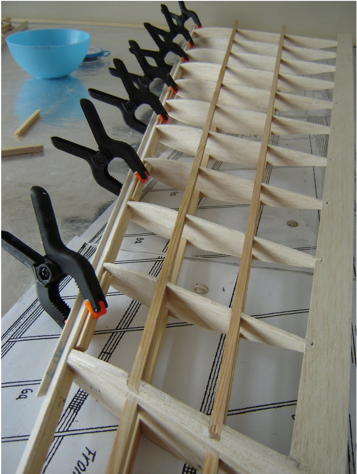
I used pieces of spruce to protect the balsa wood from being damaged by the force of the clamps.
